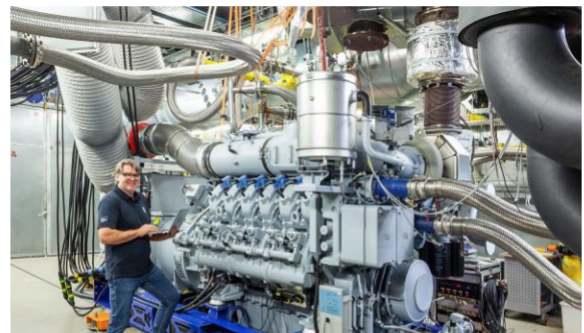
Rolls Royce Rolls-Royce's mtu Series 4000 FNER/FV Hydrogen gas engine.
