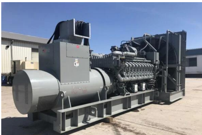
Rolls Royce MTU diesel generator
