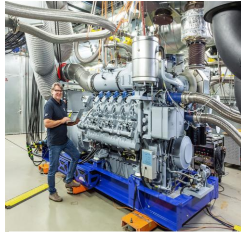
Rolls Royce Rolls-Royce's mtu Series 4000 FNER/FV Hydrogen gas engine.
